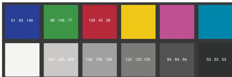
**Figure 1.2** The numbers shown here refer to a Lab space Synthetic color chart that has been converted to the Adobe RGB color space.
