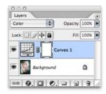
**1** Here are the steps used to create a cross-processing effect that simulates C-41 film processed in E-6 chemicals. You can adapt this technique by using different channel curve adjustments and using different fill colors. To start with I added a Curves adjustment layer which was set to the Color blend mode. I then adjusted the curves in the individual color channels as shown in the screen shots below.
