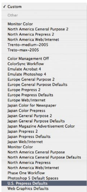
Figure 13.16 Here is a full list of the preset settings (as seen when the More Options is selected). The General Purpose presets will preserve RGB profiles, but use sRGB as the RGB work space instead of Adobe RGB. And CMYK color management will be switched off. This is a little better than the previous Web Graphics default yet may help avoid confusion among novice users. In the basic Fewer Options mode, the choice will be restricted so that all you see will be the color settings for your geographical area.
