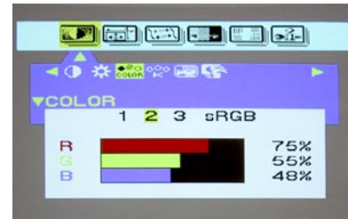
Figure 3.2 This is a screen shot showing the hardware monitor controls for the LaCie Electron blue III CRT display. The hardware controls enable me to adjust the output of the individual guns that control the red, green and blue color of the display. I adjust these settings as part of the display calibration process to make the screen neutral before building the monitor profile.
