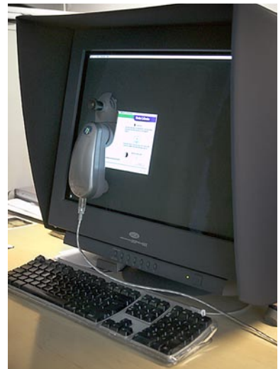
Figure 3.3 The Gretag Macbeth Eye-One is a popular spectrophotometer that can be used to accurately measure the output from the monitor display to both calibrate the output and using the accompanying Eye-One software, measure color patches, and build an ICC profile for your display.
