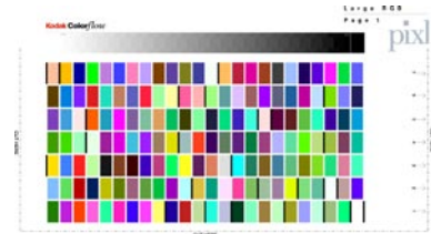
Figure 13.12 This Kodak color target can be used to construct a color ICC profile. Thomas Holm of Pixl in Denmark <th@pixl.dk> specializes in providing a custom ICC profiling service and PIXL are offering a special discount rate to readers of this book (see Appendix for more details). A profile service company will normally supply you with instructions on how to print it out. When they receive your prints, they can measure these and email the custom ICC profile back to you. For more information on printing a profile test target, refer to Chapter 14.
