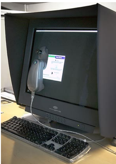
Figure 13.9 Good color management is very much dependent on having your display calibrated and profiled. This should ideally be done using a hardware calibration device like the Gretag MacBeth Eye-One system.
