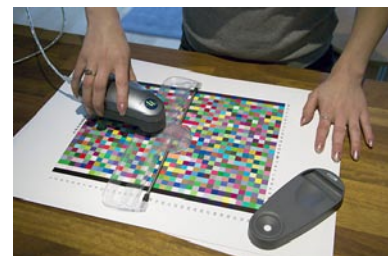
Figure 13.13 Once a print profile has been printed out, the color patches can be read using a Spectrophotometer and the measurements are used to build an ICC profile.
