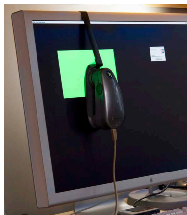
Figure 8 Good color management is very much dependent on having your display calibrated and profiled. This should ideally be done using a hardware calibration device such as the X-Rite Eye-One system.
