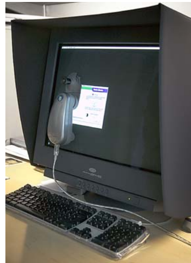
Figure 13.9 Good color management is very much dependent on having your display calibrated and profiled. This can be done using Adobe Gamma or the Apple Display calibration utility. Better still, use a hardware calibration device like the Eye-One from Gretag Macbeth.
