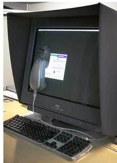
Figure 3.3 The Gretag Macbeth Eye-One is a popular spectro photometer that can be used to accurately measure the output from the monitor display to both calibrate the output and using the accompanying Eye-One software, measure color patches, and build an ICC profile for your display.
