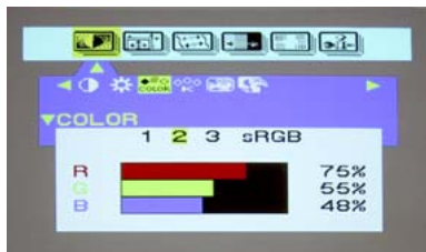
Figure 3.2 This is a screen shot showing the hardware monitor controls for the LaCie Electron blue III CRT display. The hardware controls enable me to adjust the output of the individual guns that control the red, green and blue color of the display. I adjust these settings as part of the display calibration process to make the screen neutral before building the monitor profile.
