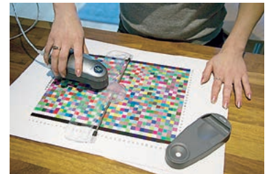
Figure 9. Once a printed profile has been printed out, the color patches can be read using a spectrophotometer and the measurements used to build an ICC profile.
