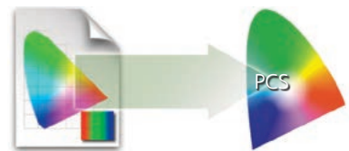
Figure 4 A color management system is able to read the profile information from an incoming RGB file and behind the scenes it builds a table that correlates the source RGB information with the Profile Connecting Space values.
