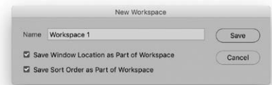
Figure 4 To create a new workspace setting, go to the Window menu and choose Workspace ⇒ New Workspace...
