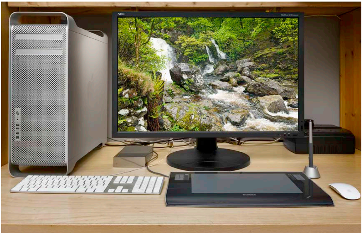
Figure 1 This shows what I might regard as an ideal basic Photoshop setup. This features a tower computer with plenty of RAM memory, a high quality calibrated display, a graphics input tablet, a removable backup drive and a UPS device to protect against power surges or cut-outs. The lighting comes from a daylight balanced tube which backlights the display. I usually have the light level turned down quite low, in order to maximize the monitor viewing contrast.
