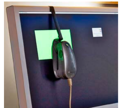
Figure 5 The X-Rite i1 Pro 2 is a popular spectrophotometer that can be used with the accompanying software, to calibrate and build an ICC profile for your display.
