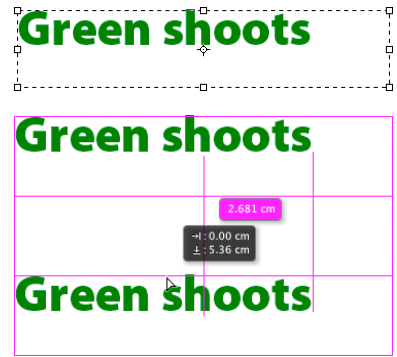
Figure 46 If you rely on Smart Guides to measure the distance between two objects it is calculated based on the distance between the object and the bounding box object. In this case it will be the distance measured between the outer bounds of the text bounding boxes.
