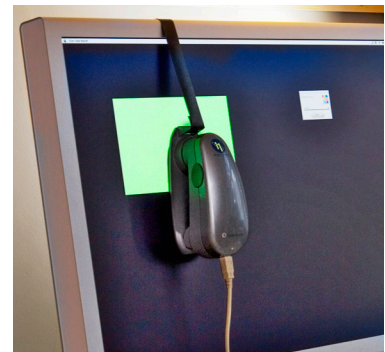
Figure 3 At work I use an X-Rite i1 Pro 2 spectrophotometer to calibrate and build an ICC profile for my displays.
